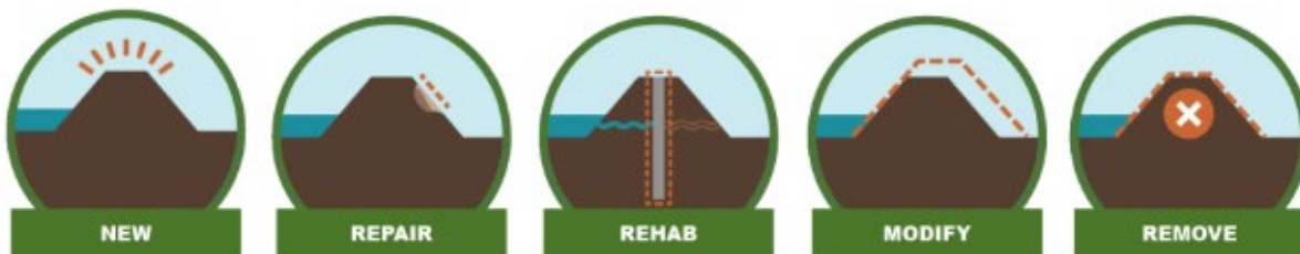
Figure 6-3: Types of Levee Projects
