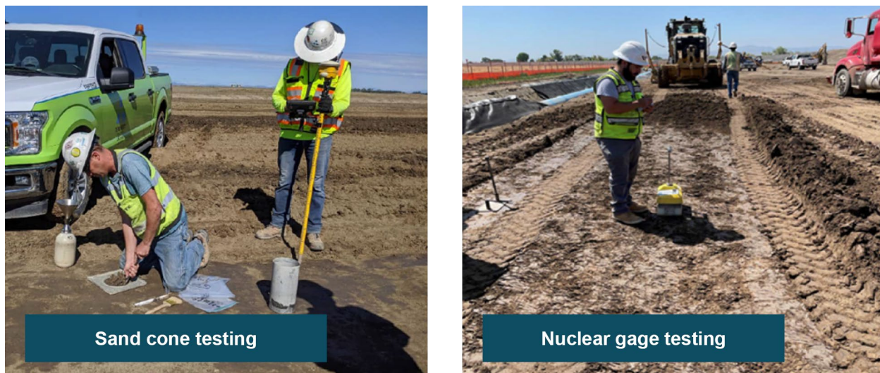
Figure 8-20: Example Density Testing
