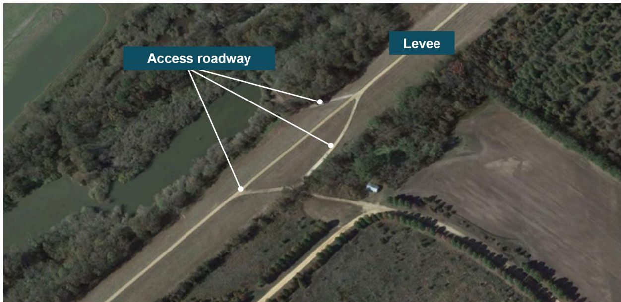
Figure 7-47: Example Access Roadway
